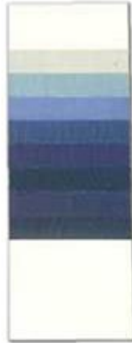
An example of a card that has been exposed to UV light and has faded.
